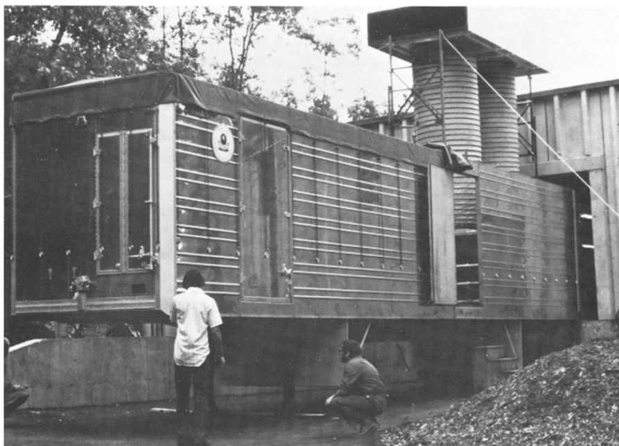
Fig 6 Dynamic reactor ("Dynactor")/separator semitrailer showing collapsible reactor column extended for use (upper right-of-center) Diesel-electric generator, control panel and bank of high-rate separators are mounted inside the trailer Nominal processing rate is 250 gal/min
