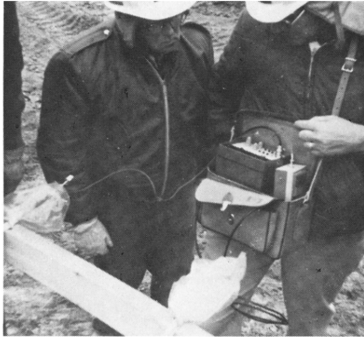
Fig 3 Closeup of acoustical emission measurement equipment showing electrical transducer (accelerometer) attached to waveguide rod (left), portable amplifier (in leather case, right), and electric pulse counter (in leather case, left)
